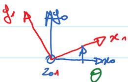
$\vec{\Omega}_\phi = \frac{d\theta}{dt} \vec{z}_{0,1} = \dot{\theta} \vec{z}_{0,1}$
