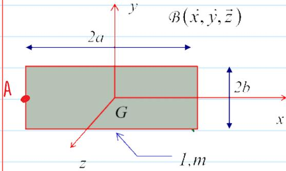
$$[I_{A,B}(s)] = \begin{bmatrix} \int_S (y^2 + z^2) dm & -\int_S xy dm & -\int_S xz dm \\ -\int_S xy dm & \int_S (z^2 + x^2) dm & -\int_S yz dm \\ -\int_S xz dm & -\int_S yz dm & \int_S (y^2 + x^2) dm \end{bmatrix}_{A,B}$$
