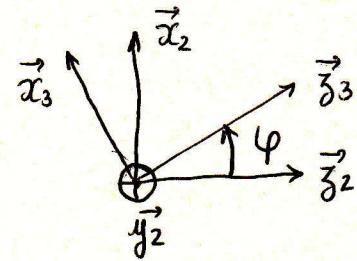
$$\vec{\Omega}(3/0) = \dot{\psi} \vec{z}_1 + \dot{\theta} \vec{x}_2 + \dot{\varphi} \vec{y}_2 = \begin{pmatrix} \dot{\theta} \\ \dot{\varphi} + \dot{\psi} \sin \theta \\ \dot{\psi} \cos \theta \end{pmatrix}_{b_2}$$
