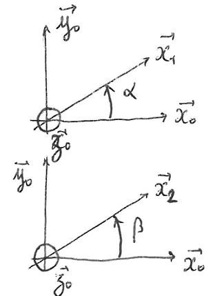
$$\vec{O_1A} + \vec{AB} = \vec{O_1B} \quad / \vec{x}_o \quad \dot{\lambda} = r \cos \alpha + L \cos \beta$$
